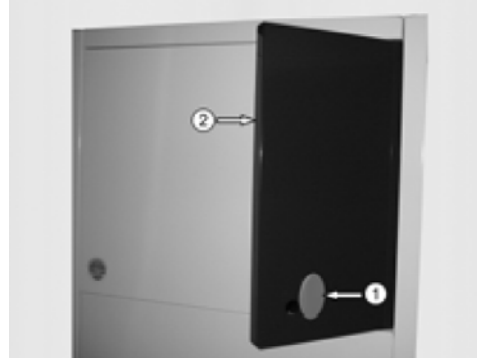
2. (1) Turn the MHG Logo, (2) insert Finger and open the cover to the right.
